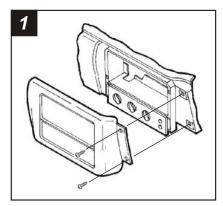
Disconnect the negative battery terminal to prevent an accidental short circuit. Open the glove box and remove (2) Phillips screws exposed on the right edge of the radio trim bezel. Unclip the bezel and remove. Remove (2) 7mm hex-head screws securing the factory head unit and disconnect the wiring.
